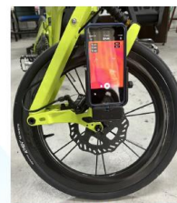
碳纖維陶瓷煞車碟盤安裝在實車上圖
